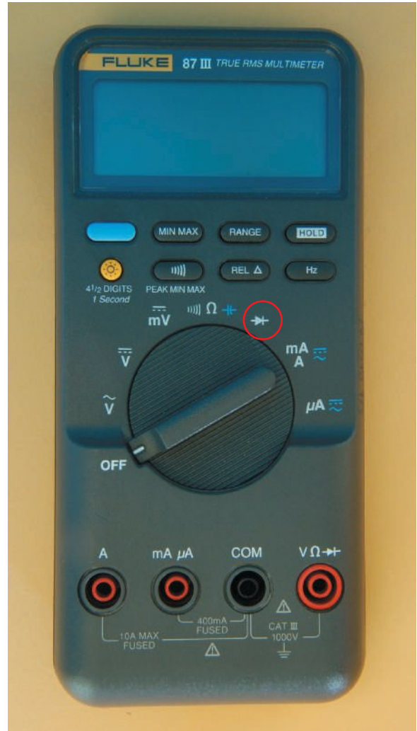
FIGURE 59-4 Meters often have a diode symbol that is used for testing semi-conductor devices.
