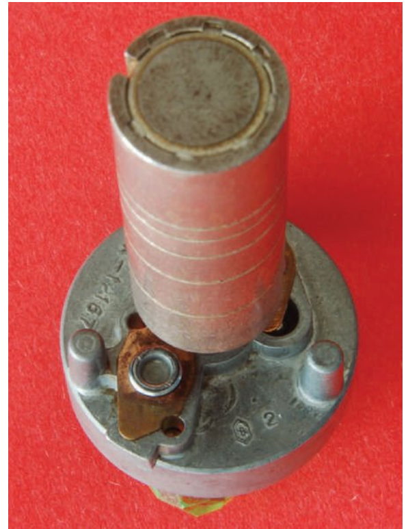
FIGURE 4-22 Setting the opening of the orifices affects the time delay of the dashpot timer.
